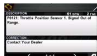
Diagnostics screen displays fault codes and suggested actions to take
