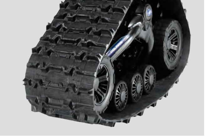
Heavy-duty, wide, rubberized wheels on a UHMW base to distribute the weight of the side-by-side
